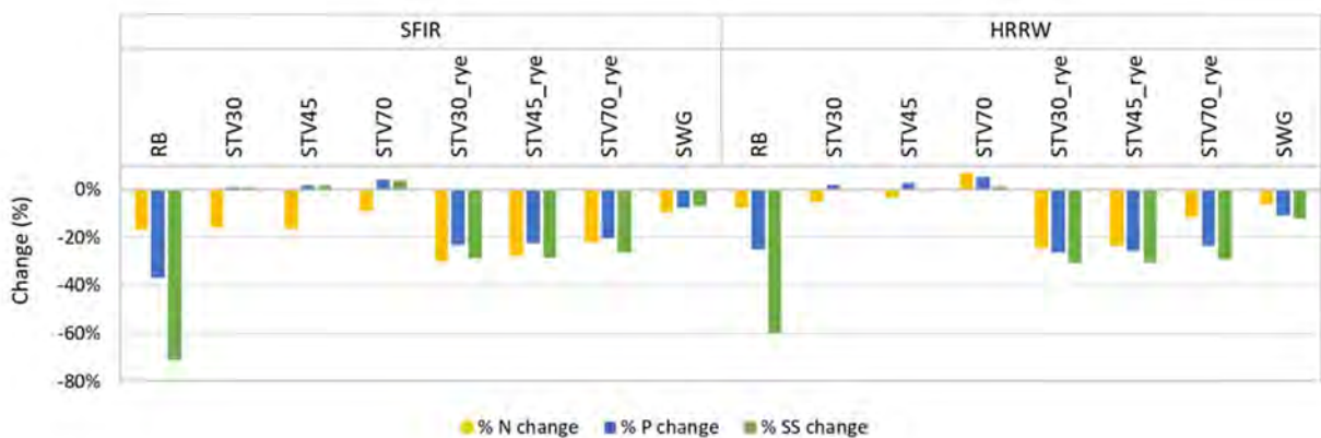
Figure 5. Impact of various bioenergy feedstock production scenarios on average N, P, and SS losses compared to baseline values at the outlet point in the SFIR or the weighted average of four HRRW sub-basins.
