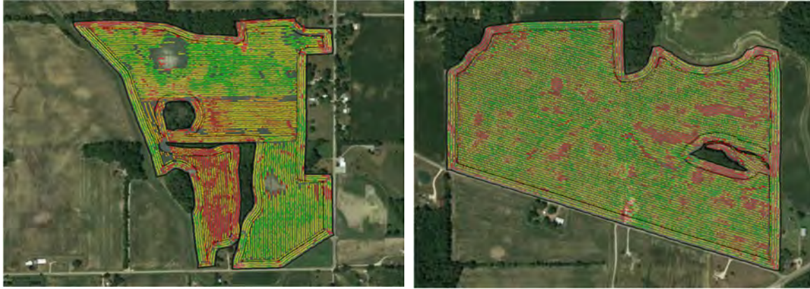
Figure 3. Harvest Map for fields with the low (Left, Field Efficiency 58.3%, Harvested Field Area 70.5 ac) and high (Right, Field Efficiency 93.7%, Harvested Field Area 92.8 ac) measured harvest field efficiencies
