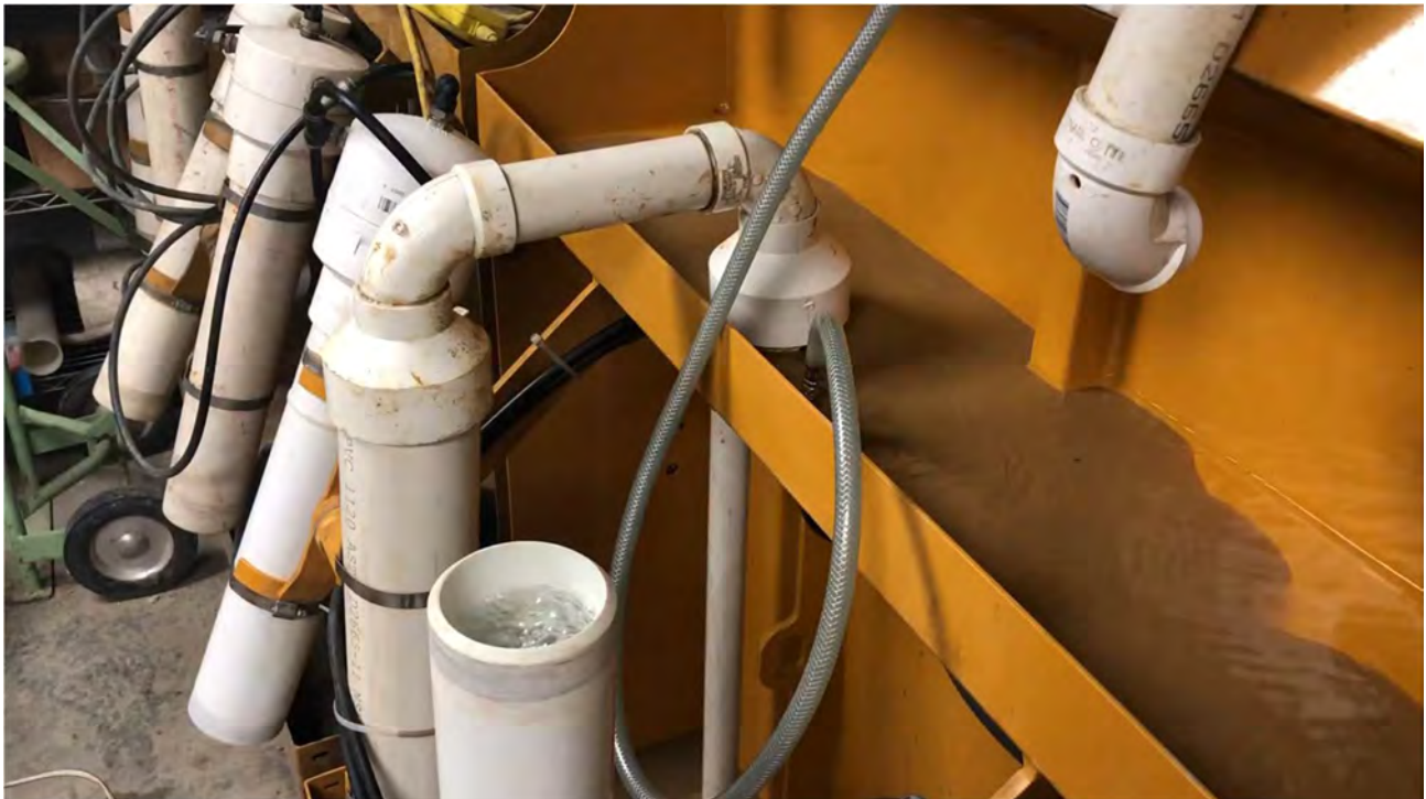
Video 1. The elutriation device used to separate root biomass from soil ( https://iastate.box.com/s/qgqnj7823r47v0ng7dhnema5kyd4gp8c )
